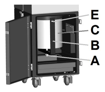
Before changing the filter cartridges hold ready an appropriate container (e.g. PE bag) for disposal.
