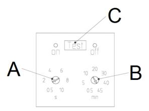
• Time interval: adjustable via controller "B".
