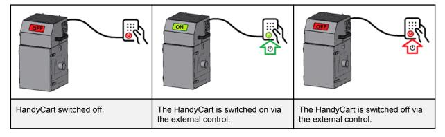
The HandyCart can also be switched off/on via its own membrane switch panel. (To this end it is necessary to separately switch on the external control.)
