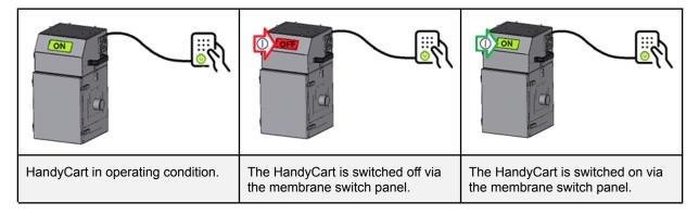
**IMPORTANT:** The HandyCart is switched on via the external control - but the HandyCart is not starting the extraction. What is going wrong?
